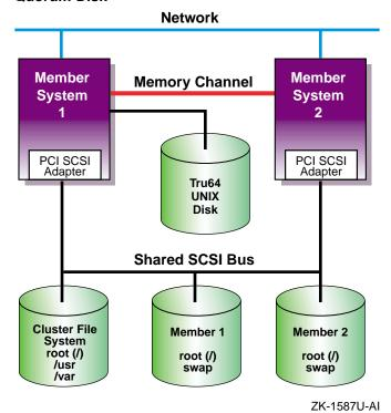
Figure 1–2 shows the same generic two-node cluster as shown in Figure 1–1, but with the addition of a quorum disk. By adding a quorum disk, a cluster may be formed if both systems are operational, or if either of the systems and the quorum disk is operational. This cluster has a higher availability than the cluster shown in Figure 1–1. See the TruCluster Server *Cluster*
